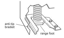
**13.** If installing the range in a mobile home, you must secure the range to the floor. Any method of securing the range is adequate as long as it conforms to the standards in the "Mobile home installation" section.
